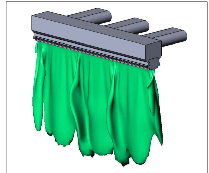
Isosurface of the velocity V=0.6 m/s AESTHETIC+BOX-STD
